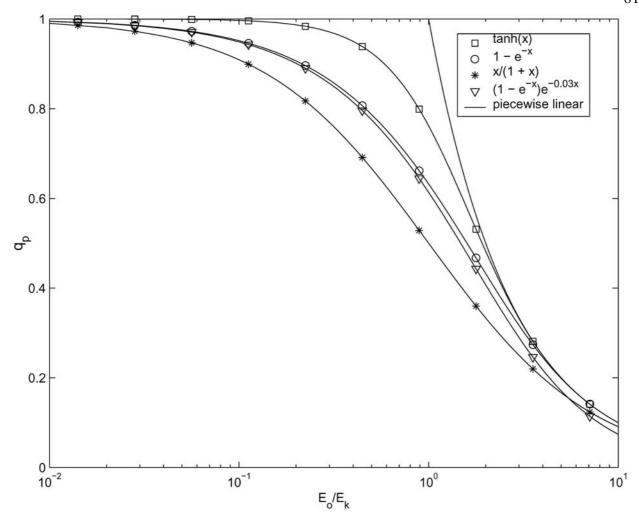
Figure 5. Expected relationship between  $q_p$  and  $E_o/E_k$  for model equations 4-8.
